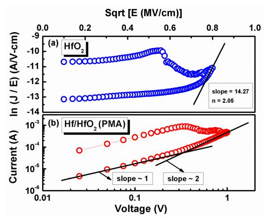
**Figure 2**. Curve fitting in Pt/HfO<sub>2</sub>/TiN devices (a) Poole-Frenkel emission and in Pt/Hf/HfO<sub>2</sub>/TiN devices (b) SCLC mechanism.
