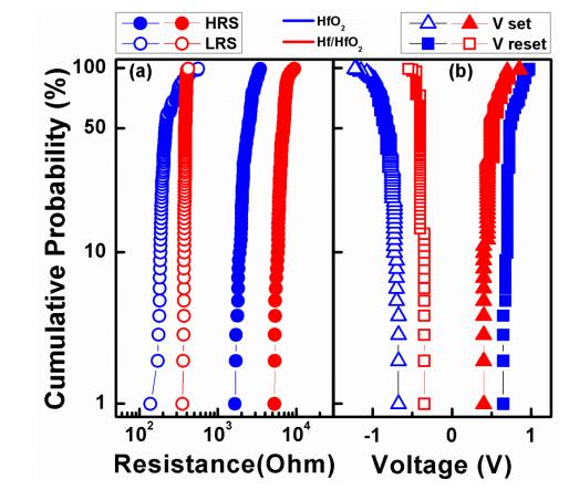
**Figure 5.** Statistical distribution of resistive switching parameters during 100 continuous cycles in both Pt/HfO<sub>2</sub>/TiN and Pt/Hf/HfO<sub>2</sub>/TiN devices. (a) HRS and LRS. (b) V<sub>set</sub> and V<sub>reset</sub>.
