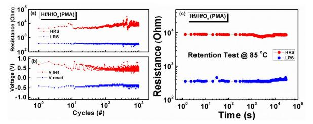
Figure 6. The  $10^3$  stable endurance cycles of the Pt/Hf/HfO<sub>2</sub>/TiN device: (a) HRS and LRS. (b)  $V_{set}$  and  $V_{reset}$ . (c) Data retention characteristics at 85 °C under 100mV stress.
