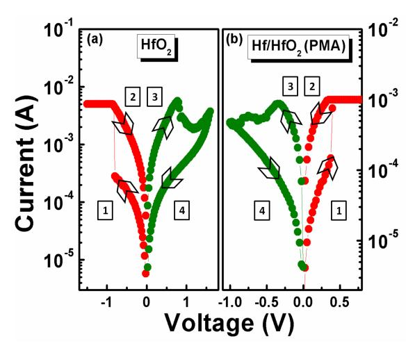
Figure 1. Reverse polarity operation in resistive switching between Pt/HfO2/TiN and
